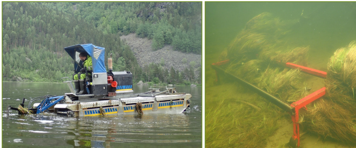
Figure 3. Mechanical management methods of aquatic macrophyte mass developments. Mechanical cutting by boat (left) and scraping with a harrow to remove plant roots (right). Both examples from removal of Juncus bulbosus in the Rysstad Basin, River Otra, Norway.
